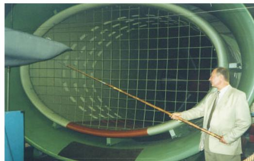
Drag coefficient of yunibus —  $C_x = 0.079$  (sports car is 0.34). This will reduce the required drive power of 40-seat yunibus, for example at a speed of 450 km/hour, at 1800 kW.
